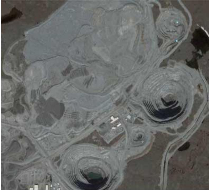
*Aerial photo of the Ekati mine showing two large open pit mines, with a smaller pit in between and another near the top of the photo.*
