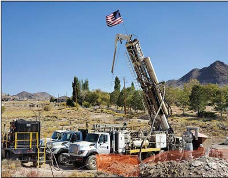
*Here is a reverse circulation percussion drilling rig set up and drilling in west Tonopah. This type of drilling yields small chips and sands for assay testing and is fast and lower cost.*
