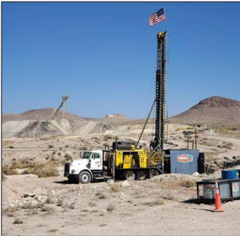
*A core drilling rig working in west Tonopah on the Blackrock gold property. Core drilling is more expensive than percussion, but it yields a complete slice of the vein.*
